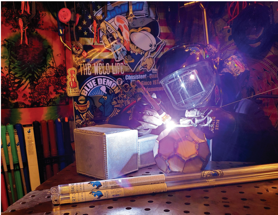
Fig. 1 — Sean Flottmann prefers GTAW and stainless steel. For practice here, he performed GTAW to join several six-sided pieces of stainless steel into a soccer-ball sculpture. “You don’t want your skills to be static,” he said. Oversized cubes he crafted can also be seen.
