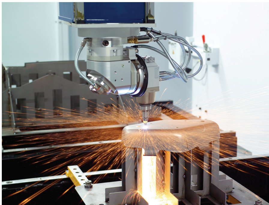
High-quality laser cutting results from the optimal combination of a series of cutting parameters, including laser power, focus, speed, gas pressure, and piercing strategy.
