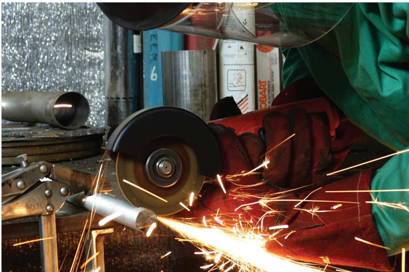
Fig. 1 — Maximizing productivity and quality when cutting metal with a right-angle grinder depends on many factors, including choosing the right abrasive and using it properly.
