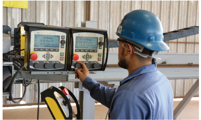
Fig. 4 — An operator controls SAW parameters using a digital controller and handheld pendant.
