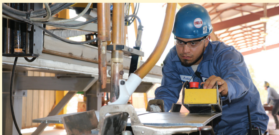
Submerged Arc Welding Operator Justin Montemayor centers the electrode within the joint and adjusts the torch height.
